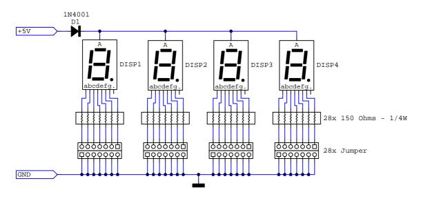
Displays are 0.5" high 7-segments with Common Anode Use displays with 10 pins, located on upper and lower side of the display
