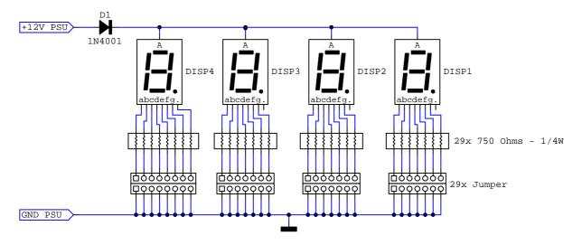
Displays are blue 0.56" 7-segments with Common Anode as manufactured by Liteon (LTS-5501AB)
